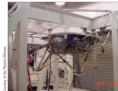
■ FIGURE 6–58 This 2005 photo shows the lander of the Phoenix Mission to Mars suspended in the hot-fire test bed at Lockheed Martin Space Systems in Denver.
